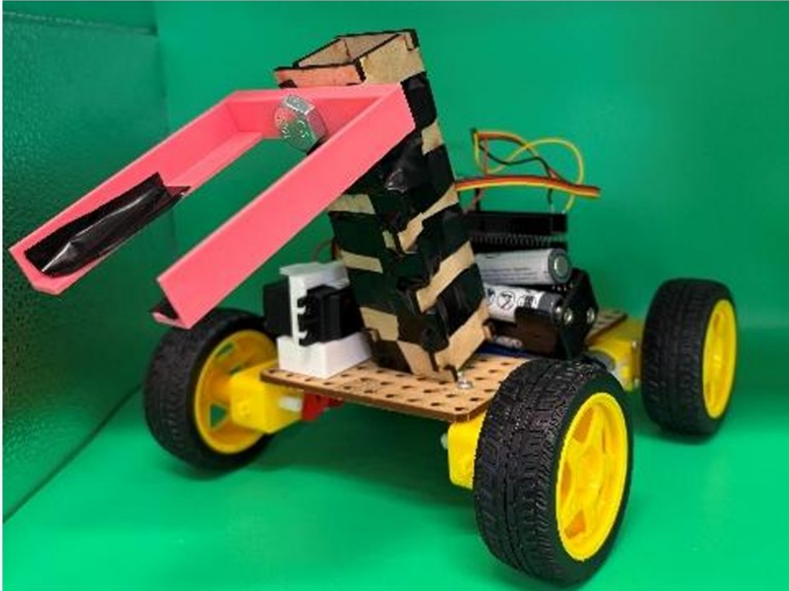
Earlier rescue-arm prototype: pickup geometry and alignment were unreliable.
